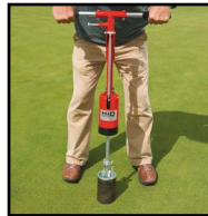
2. Remove pin. Lift handle and hammer actions drives cutter into the ground.
